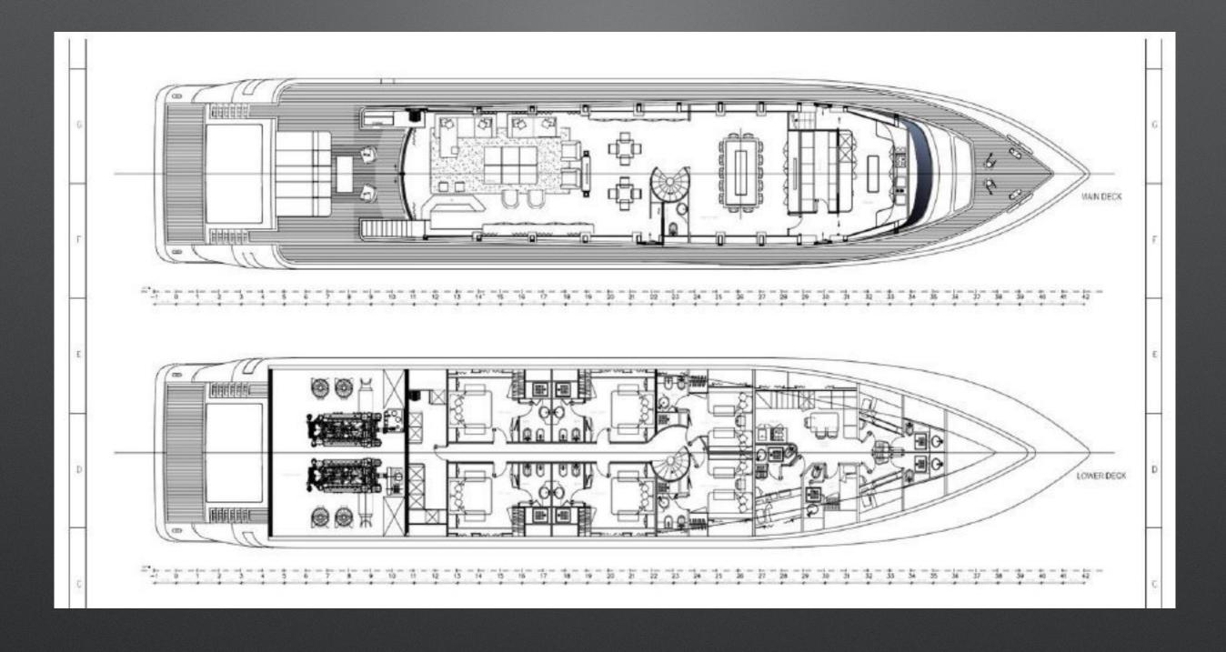
**BUILDER:** Admiral Tecnomar **YEAR**: 2010 **REFIT:** 2017/2018/2020 New Paint FLAG: Italian **ACCOMMODATION**: 7 cabins for 16 guests LOA: 44 meters **BEAM**: 8,5 meters **SPEED**: 15 Low Cons. / 25-27 Max **MATERIAL:** Reinforced Composite Fiber Glass **ENGINES**: 2 x 4000 Hp MTU **SEAKEEPER**: Zero Speed Stabilizers
